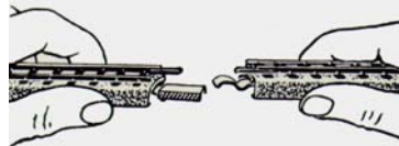
Fig. 10 Fitting the center conductor insulator 5022
